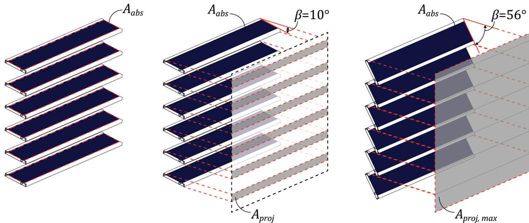
FIG. 6 Different areas that can be used as reference area  $A_{ref}$  to calculate the solar thermal efficiency  $\eta$ . Left: Overall slat absorber area  $A_{abs,tot} \approx 2.67 \text{ m}^2$ . Centre: Projected slat area  $A_{proj}$  for exemplary slat tilt angle of  $\beta = 10^\circ$ . Right: Maximum projected slat area  $A_{proj,max} = 3.15 \text{ m}^2 \cdot BE$  for slat tilt angles of  $\beta \geq 56^\circ$ .
