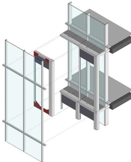
FIG. 8 STVB installation in Scenario 1 on a multi-storey ventilated double-skin façade
