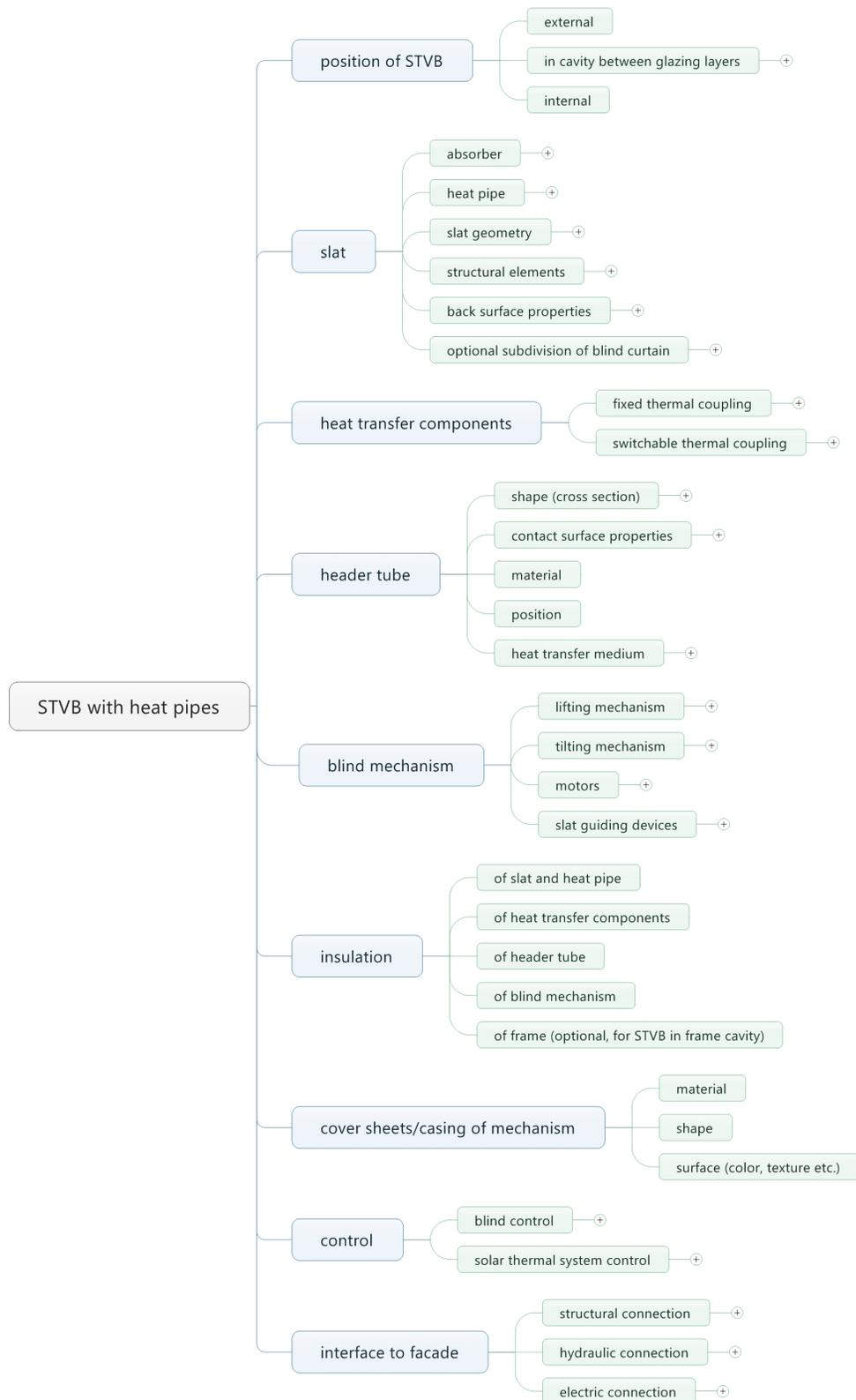
FIG. 2 First and second level of the design parameter space of solar thermal venetian blinds with heat pipes. The full design parameter space is provided as a supplementary file.
