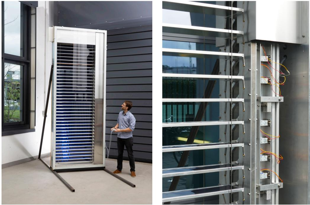
FIG. 5 Left: Test sample of double skin façade element (1.4 m x 3.6 m) with integrated solar thermal venetian blind seen from the exterior side. Right: Switchable thermal coupling mechanism with springs and solenoids mounted in the test sample, upper part covered with cover sheets.
