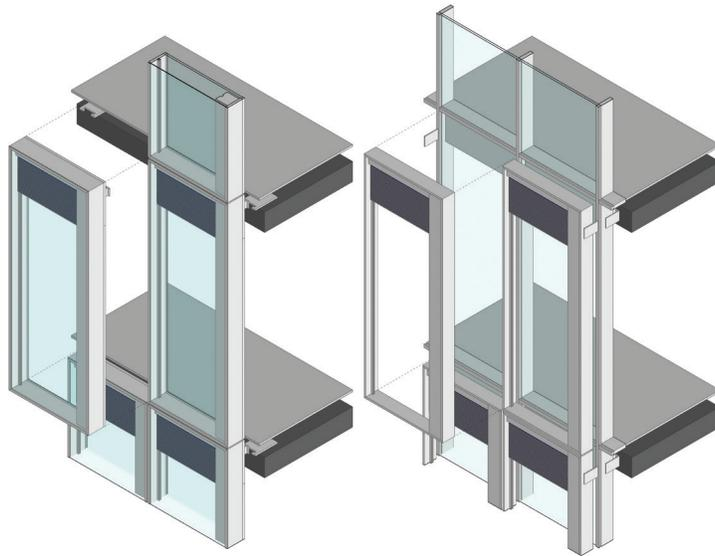
FIG. 9 STVB installation in Scenario 2 as part of double skin unitised façade (left); as an additional stand-alone element on an existing unitised or stick façade system (right)
