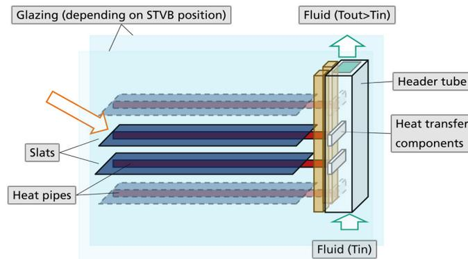
FIG. 1 Main components of a solar thermal venetian blind positioned between an outer and an inner glazing pane. The increase between fluid inlet temperature  $T_{in}$  and fluid outlet temperature  $T_{out}$  illustrates the harvesting of solar thermal heat. The blind mechanism for retracting and tilting the slats is not shown.
