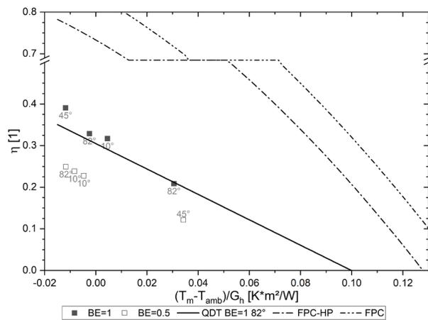
FIG. 7 Efficiency curves  $\eta$  of STVB test sample for  $T_{int} \approx T_{amb}$  as function of mean fluid temperature  $T_m$ , ambient temperature  $T_{amb}$ , and hemispherical irradiance  $G_h$  compared to reference collectors (cf. TABLE 3). Slat tilt angles  $\beta$  noted as label for each data point. Reference area  $A_{abs,total} = 2.67 \text{ m}^2$  used for the STVB.
