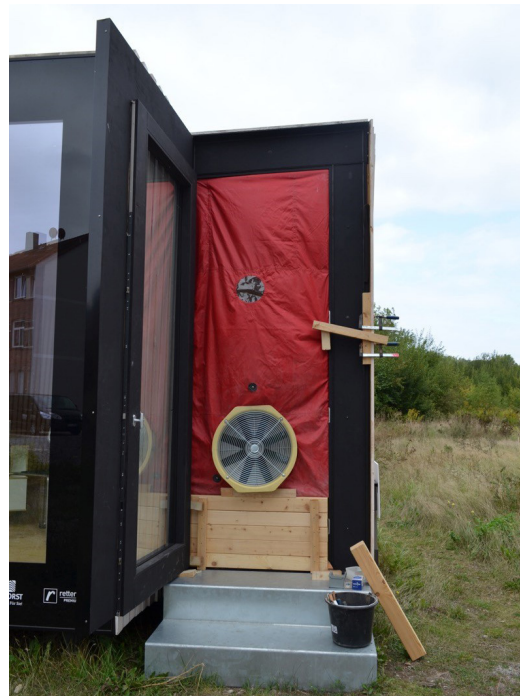
FIG. 7 IBA: Timber Prototype House blower-door test
