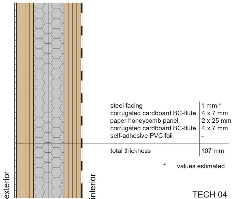
FIG. 11 TECH 04 envelope section Tube Envelope
