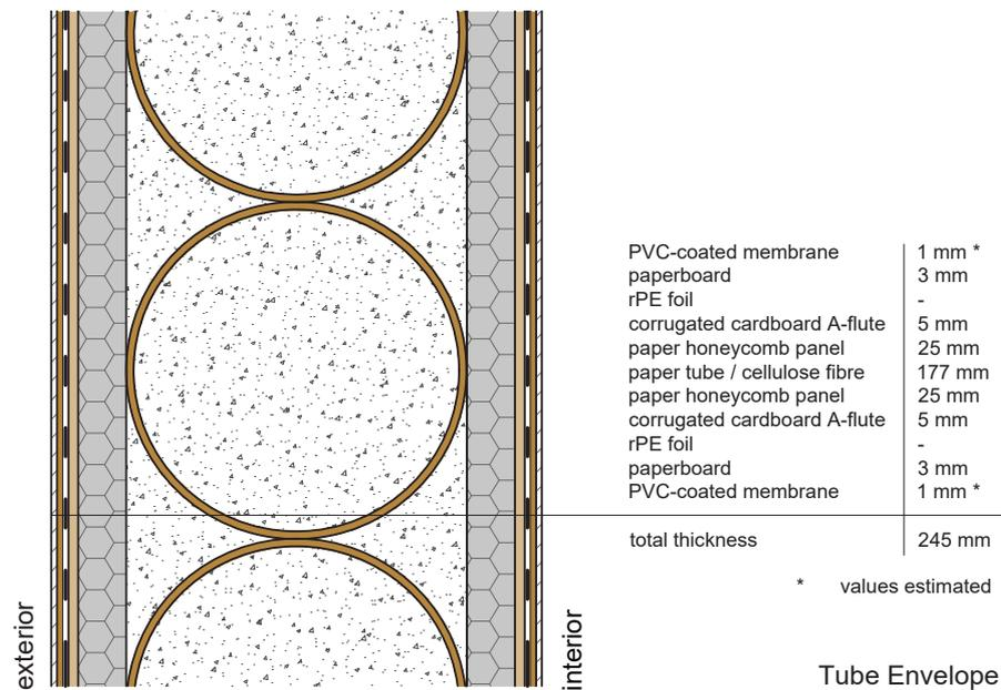
FIG. 13 Tube Envelope section
