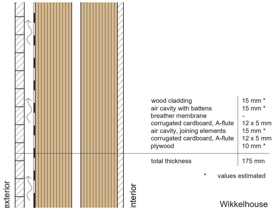
FIG. 7 Wikkelhouse envelope section
