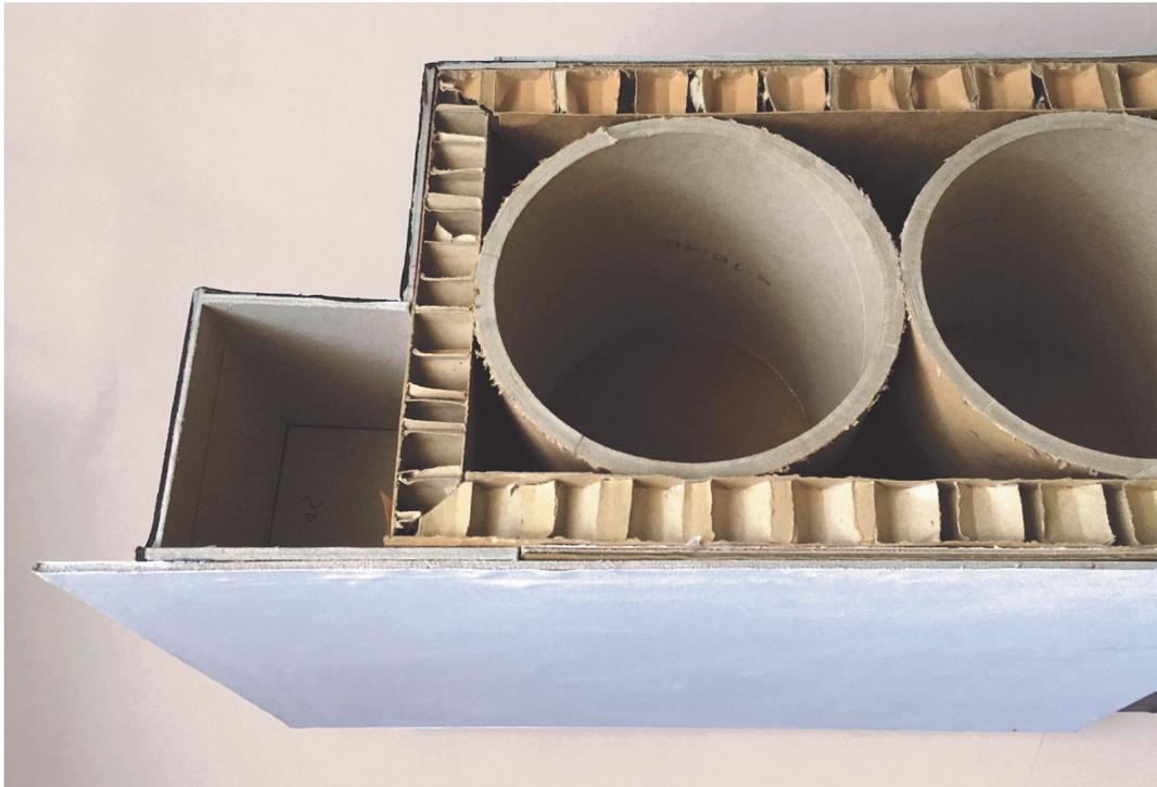
FIG. 12 A prototype of the Tube Envelope panel
