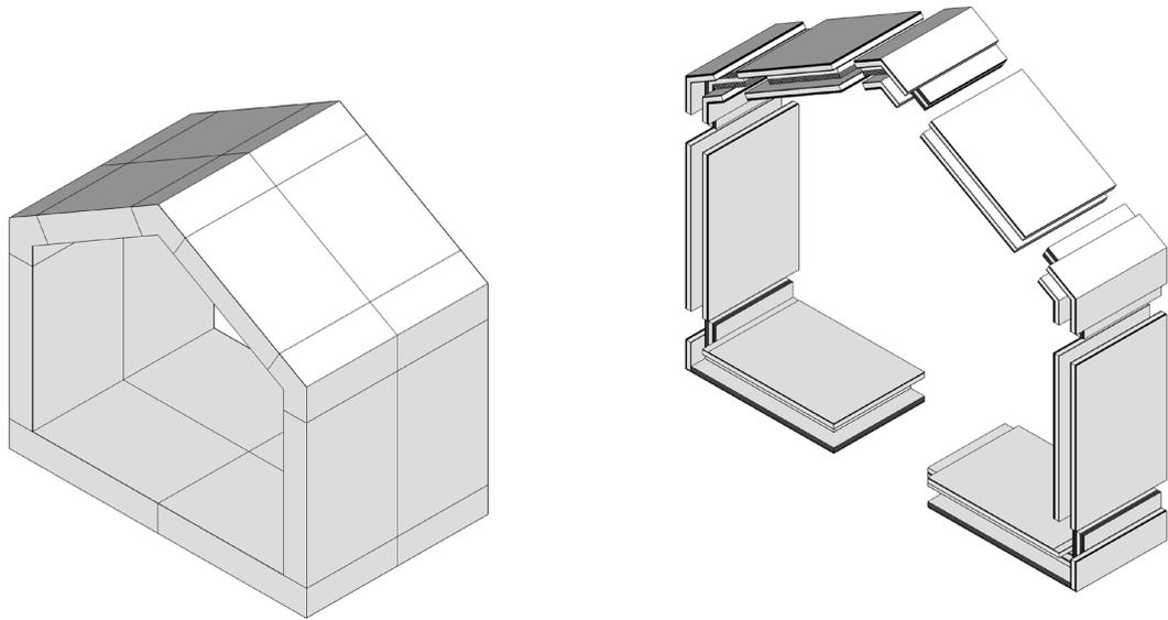
FIG. 4 Construction principle for the demonstrator of the paper emergency shelter
