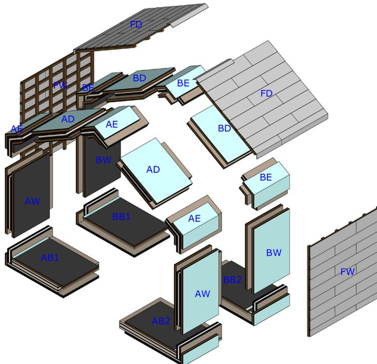
FIG. 6 Exploded view of the demonstrator
