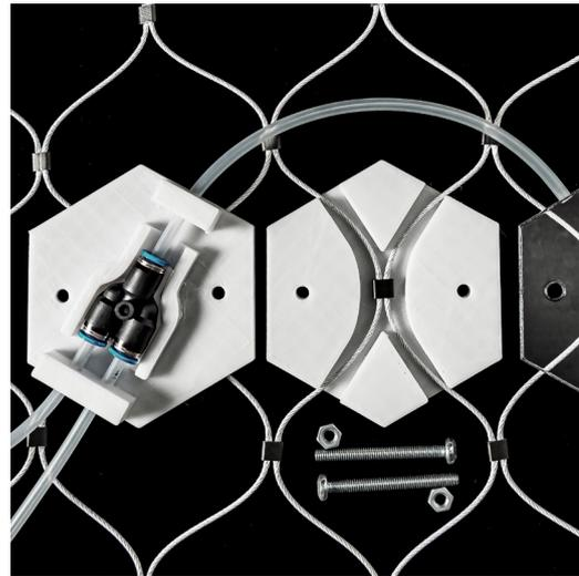
FIG. 10 Connection joint for PAOSS elements.
