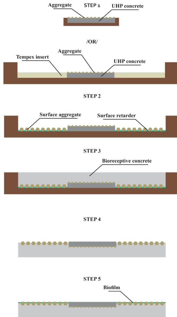
FIG. 3 Graphical overview of the panel production process
