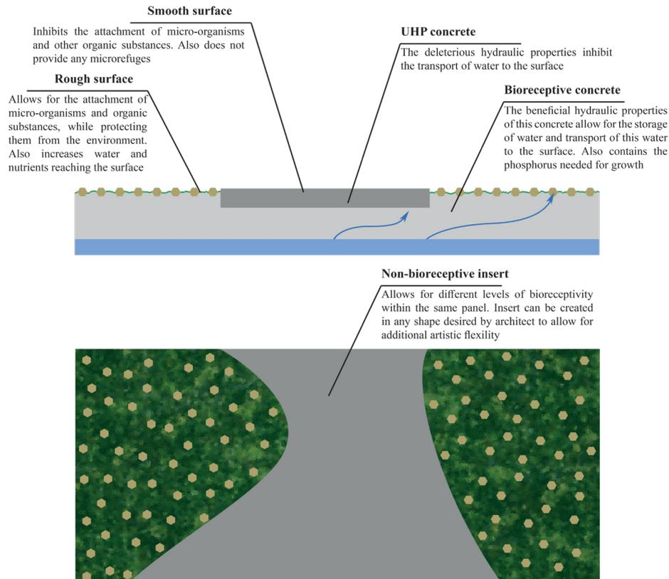
FIG. 2 Overview of the final panel design
