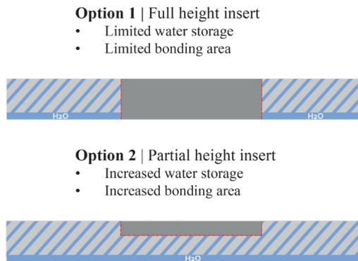
FIG. 1 Sectional overview of different insert options
