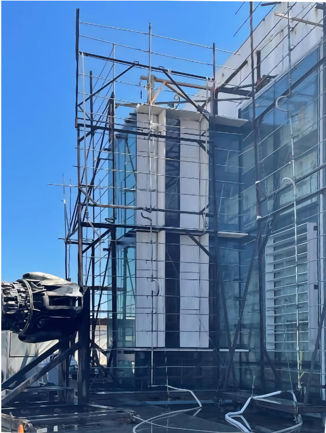
FIG. 8 Performance mock-up: Dynamic air and water infiltration is tested by using a wind turbine to generate dynamic wind loads.
