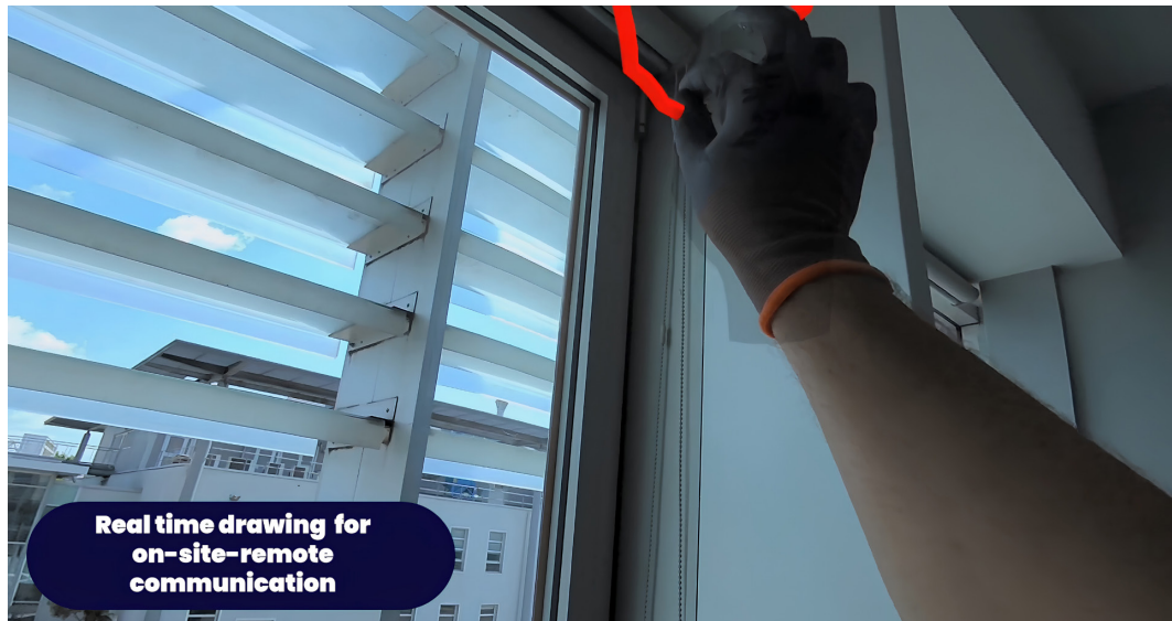
FIG. 5 Visor XR platform functionality: real-time drawing for easy communication with remote technicians. Picture from the visor used by the operator.
