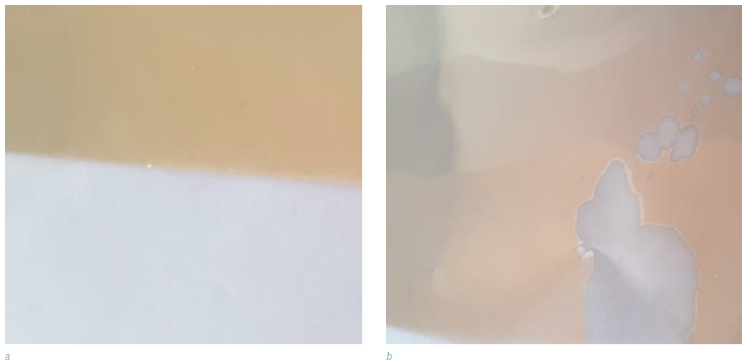
FIG. 8 a) Selective, metallised ETFE film against white background – b) Degraded coating after severe environmental stress: temperature, strain, condensate (source: author)
