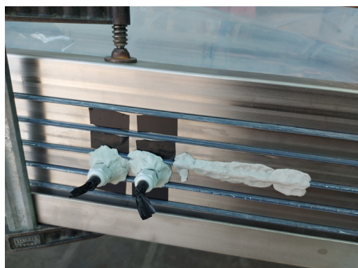
FIG. 23 Sealing improvement at distinct leakage points after the mock-up entered service
