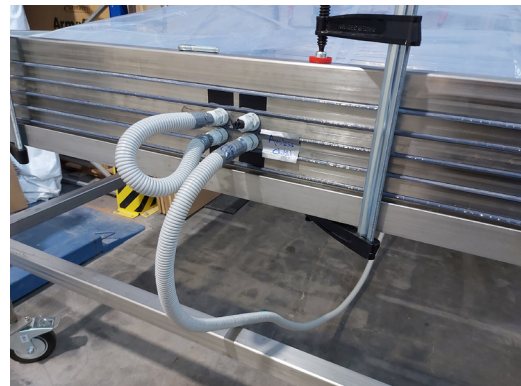
FIG. 15 Interconnecting the four air chambers of the mock-up using by-passes, forming 2 air chamber-groups
