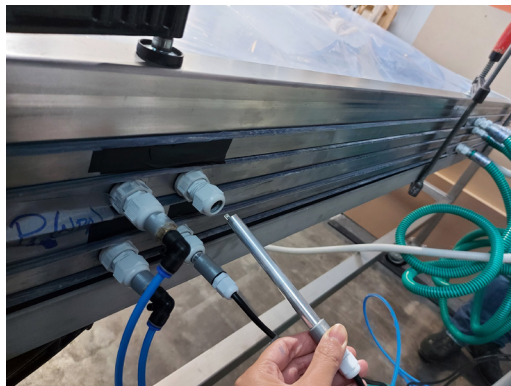
FIG. 14 Different sensors connected to the air chambers of the Mock-Up through the holes all around the frames: The blue hoses are sampling the air of each air chamber to the pressure sensors, the black cables connect the temperature sensors, and green hoses transfer the airflow between the air chambers and the air supply system
