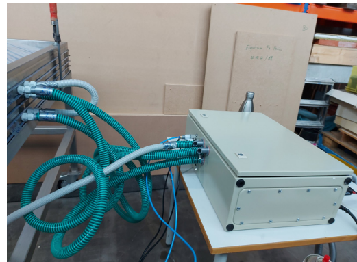
FIG. 17 The control box is connected to the mock-up on the left side, and the air supply system is directly connected on the right side
