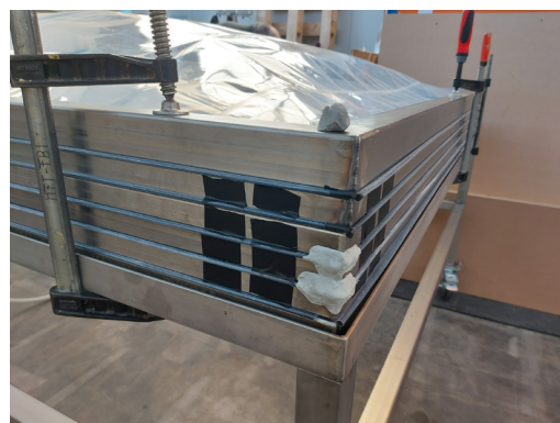
FIG. 24 Sealing improvement at distinct leakage points after the mock-up entered service
