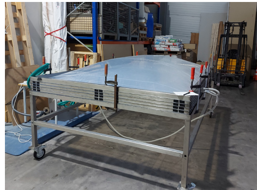
FIG. 13 The mock-up after full assembly in the lab: Air chambers are filled with air (inflated)
