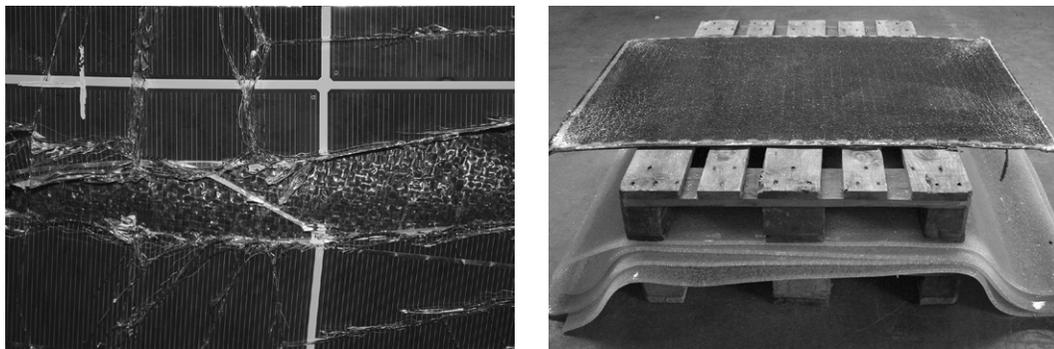
FIG. 6 Improved residual resistance due to PV wafer cells' soldered interconnectors (left, here: at  $+68 \text{ }^\circ\text{C}$ ) and flexible PV thin-film cells stiffening the broken laminate (right, here: in contrast to LSG made of TTG without integrated PV layer)
