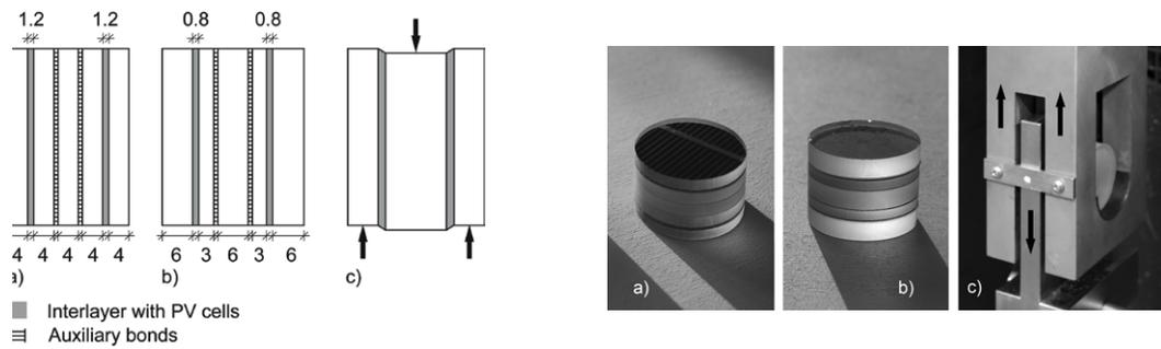
FIG. 3 Shear test specimens incorporating a) PV wafer cells or b) flexible CIGS cells and c) test set-up and apparatus
