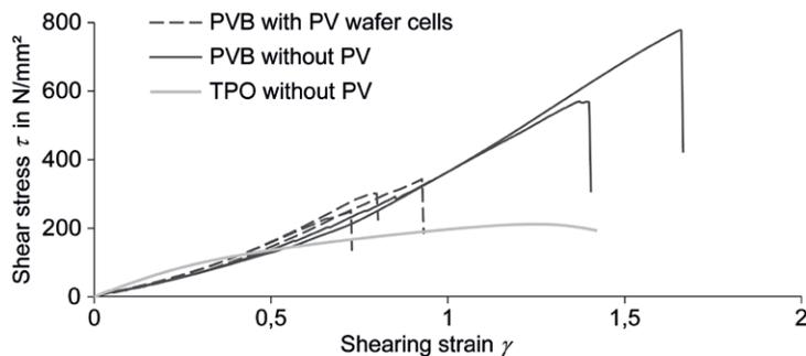
FIG. 7 Shear stress to shear strain diagram at +22 °C and 30.7 % relative humidity
