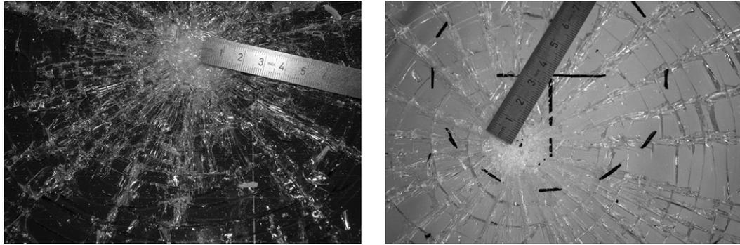
FIG. 4 Larger amount of loose glass splinters on the PV-coated superstrate glass (left) compared to the uncoated LSG cover glass (right) at the point of impact after ball drop
