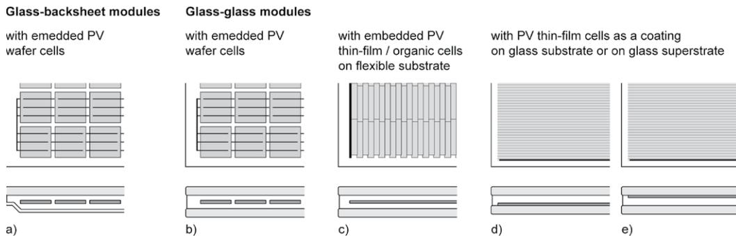
FIG. 2 Views and sections of common types of PV modules
