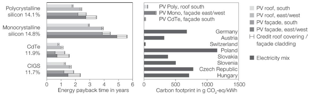
FIG. 8 Energy payback time depending on PV technology and BIPV application in Central Europe and carbon footprint in comparison with country electricity mixes
