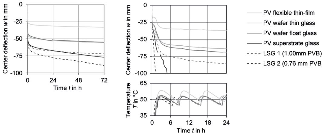
FIG. 5 Mean values of the measured centre deflections in the standard scenario (test load  $0.65 \text{ kN/m}^2$  at room temperature, left) and in the increased temperature scenario (test load  $0.325 \text{ kN/m}^2$  at  $+50 \text{ }^\circ\text{C}$ )
