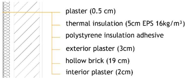
FIG. 3 Section of existing building wall assembly
