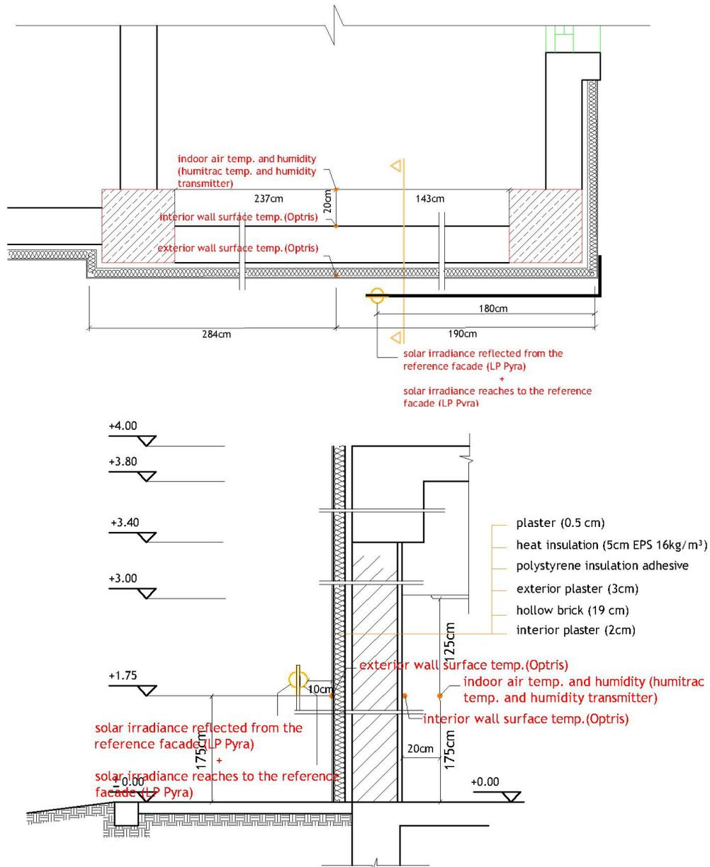
FIG. 5 Sections and plans of experimental setup of reference facade
