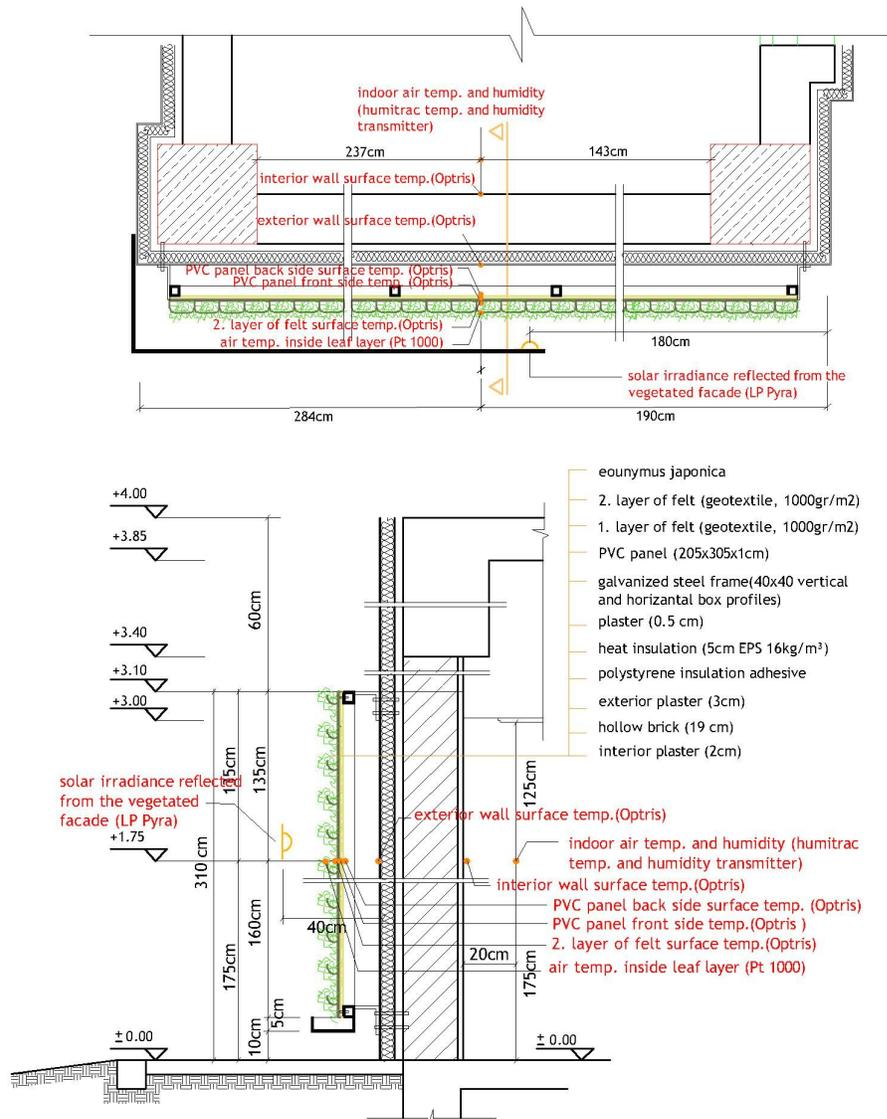
FIG. 4 Sections and plans of experimental setup of vegetated facade
