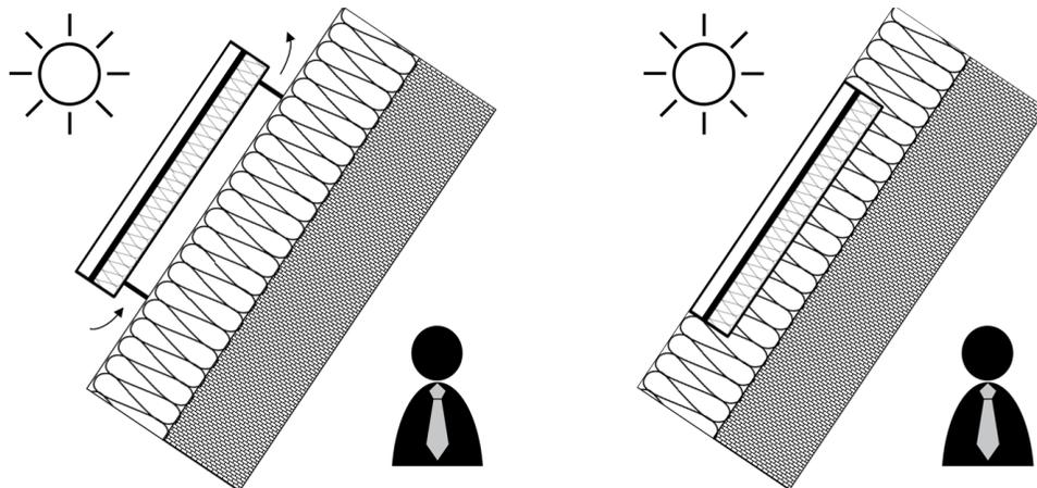
FIG. 1 Schematic drawings of a building-added solar thermal collector (left) and building-integrated solar thermal collector (right)
