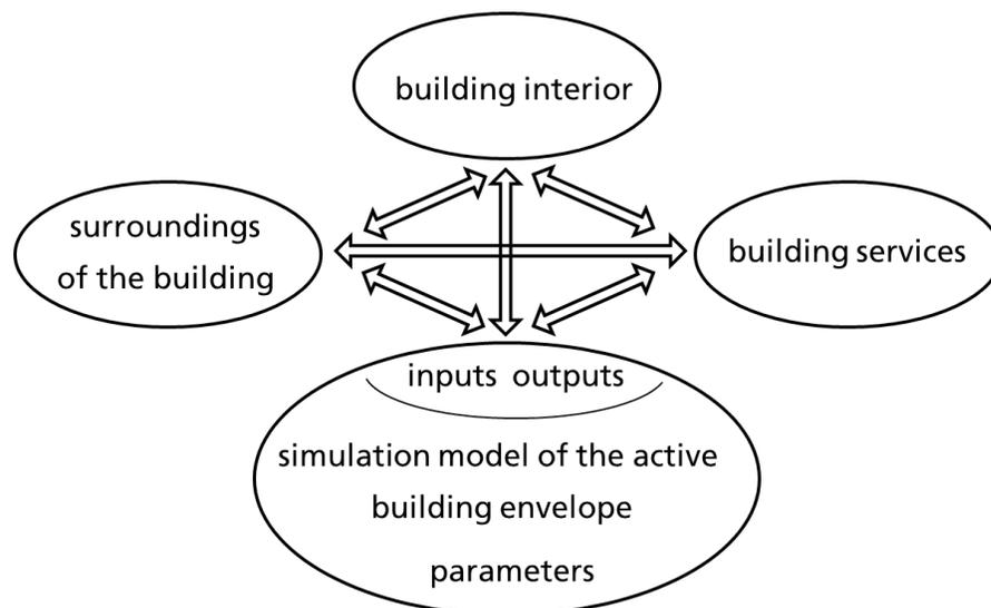
FIG. 2 Schematic drawing of the links between the simulation model of an active building envelope and the surroundings, the interior, and the building services of the building.
