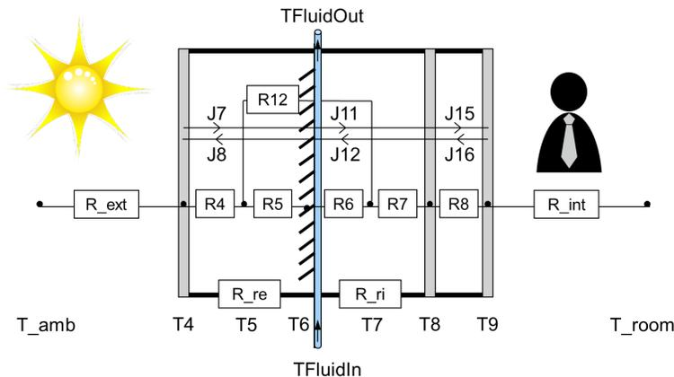
FIG. 3 Schematic drawing of a detailed physical model of a semi-transparent solar thermal facade collector with the average temperatures of the surroundings,  $T_{amb}$ , of the layers of the facade T4 to T9, the temperature of the interior,  $T_{room}$ , and the fluid inlet and outlet temperature,  $T_{FluidIn}$ , and,  $T_{FluidOut}$ . R indicates the thermal resistances between the layers, and J represents the infrared radiation within the element
