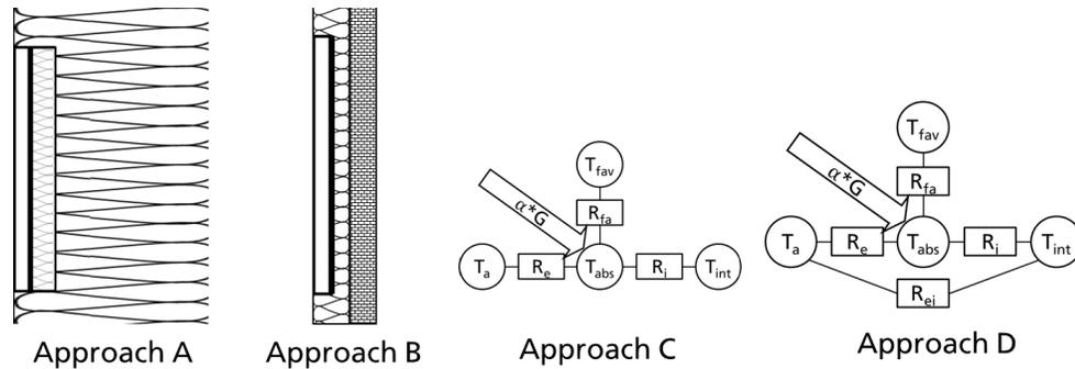
FIG. 4 Schematic illustration of the four simple approaches to model BIST
