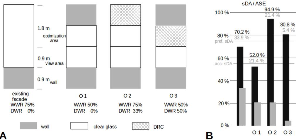
FIG. 5 Schematic layout of the existing facade and three optimization variants (A). Bar diagram showing sDA (black) and ASE (grey) for the existing facade and the three optimization variants O1-O3 (B).
