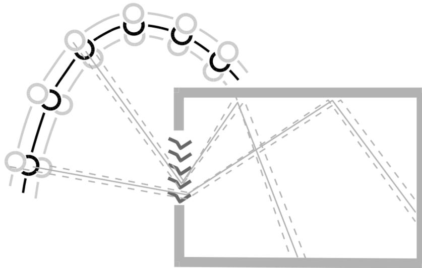
FIG. 2 Shared Sun Path concept: coefficients calculated for one day sequence (black sun positions, solid light rays) can be used for a few days before and after the calculation day (grey sun positions, dashed light rays)
