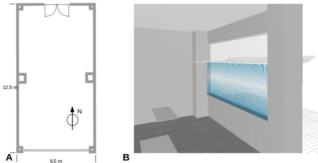
FIG. 7 Classroom with south-facing facade used for the project work (A) and combined interior and exterior light shelf with upward bent shape (B)
