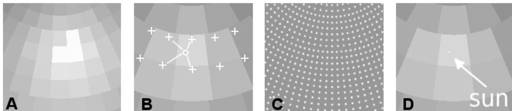
FIG. 1 Sun coefficient models: RADIANCE 3 Phase Method (A, with subdivision factor 2), DAYSIM (B), RADIANCE 5 Phase Method (C), EvalDRC (D). Only a section of the sky hemisphere is shown.
