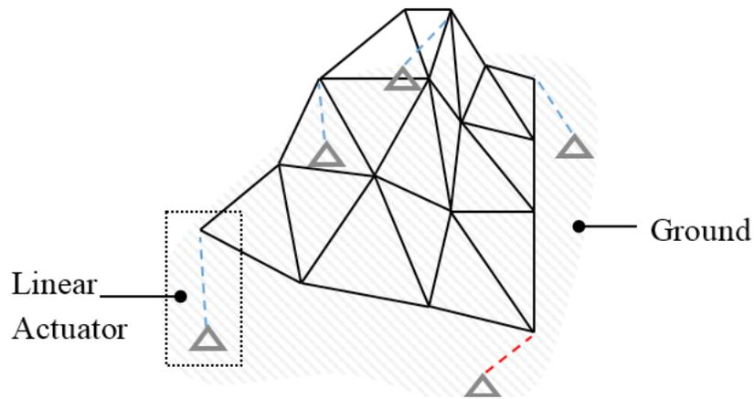
FIG. 5 Scheme of an adaptive envelope linked to a supporting structure by linear actuators. Actuators are pin-jointed both to the supporting structure and to the envelope.
