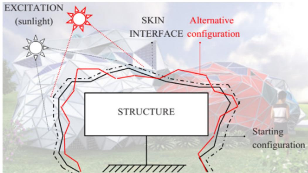
FIG. 1 The “building skin” as the interface to non-structural design drivers (e.g. sunlight).
