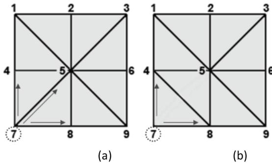
FIG. 6 (a) and (b): two frameworks with the same number of nodes and edges but with a different pattern topology. In (b) node 7 has connectivity  $\leq 2$  and needs to be controlled directly.
