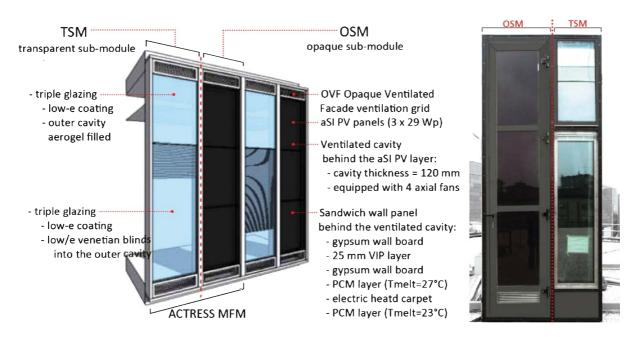
Fig. 5. The ACTRESS prototype (left) and a sketch of the various components (right).
