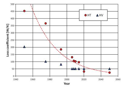
**Fig. 3.** Transmission and ventilation loss coefficients versus time for a typical residential building (100 m<sup>2</sup> of floor area, window area 1/8 of the floor area.  $H_T$  = loss coefficient for transmission,  $H_V$  = loss coefficient for ventilation).
