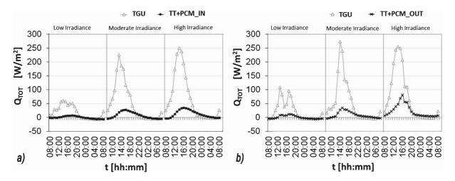
Fig. 10. Time profiles of total heat flux - TT+PCM\_IN and reference (a) and TT+PCM\_OUT and reference (b).
