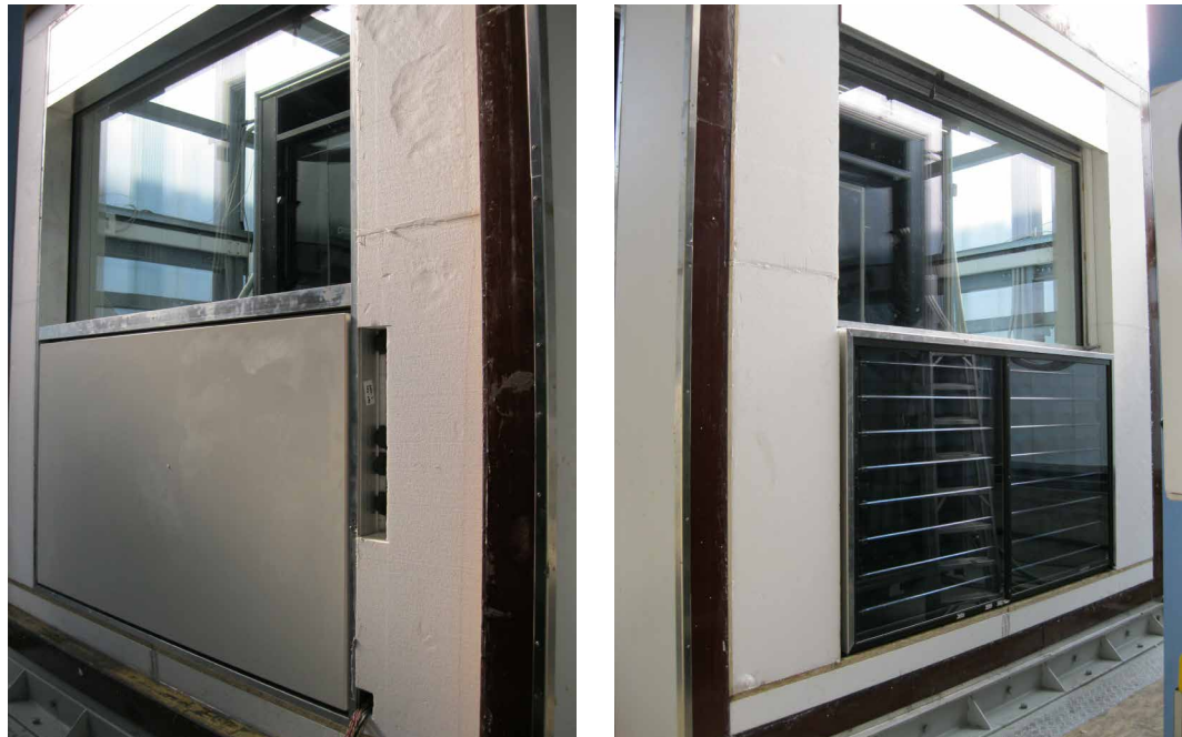
FIG. 2 View from inside (left) and outside (right) of façade prototype taken during the tests in the climatic chamber.
