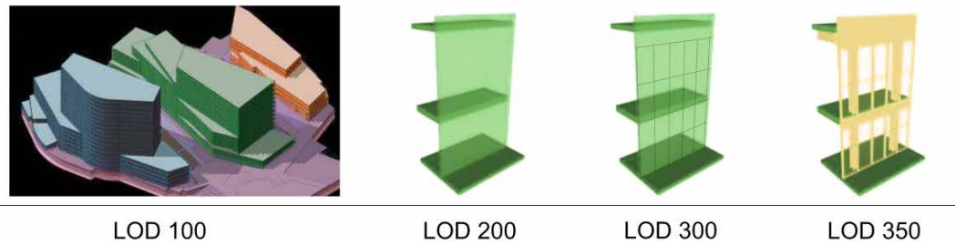
FIG. 4 Level of development of a curtain wall system. (Image by BIM forum)
