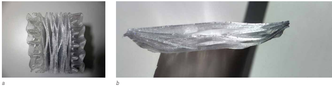
FIG. 3 Cross section of the panels, showing the elongated cells in the insulation core and the channels in the external water layer.
