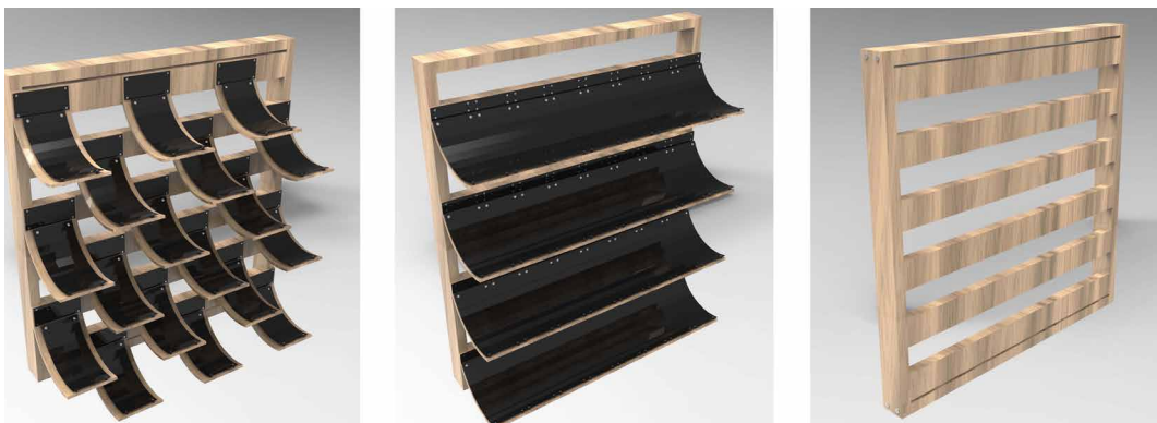
FIG. 13 Renders of 15x10cm (on the left) and 15x60cm lamellae panels (on the centre). Wooden panel substructure detail (on the right)
