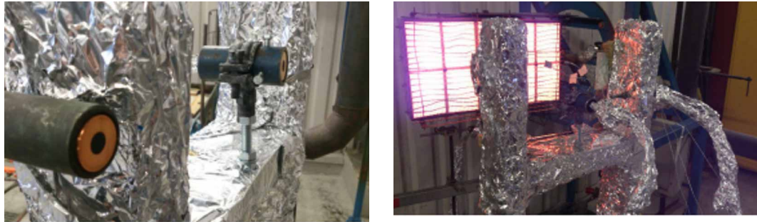
FIG. 2 Radiant panel tests (debuyser, 2015; Debuyser et al., 2017) (left); heat flux meters mounted on the frame, (right) testing of a sample
