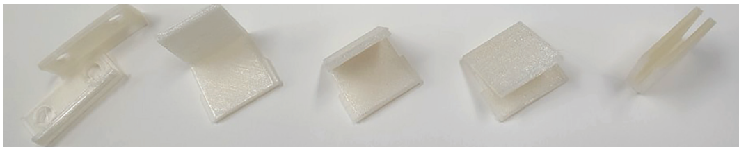
FIG. 6 Programming of rotating angles by 3d printing the customised angled hinges
