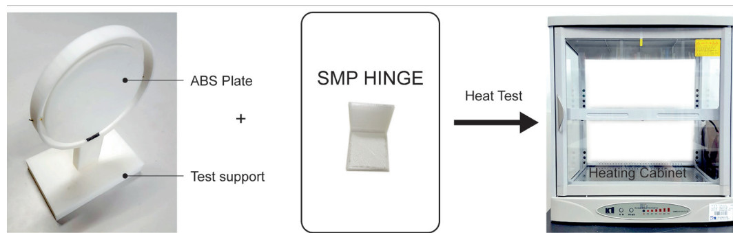
FIG. 7 Baseline prototype and heat test setup
