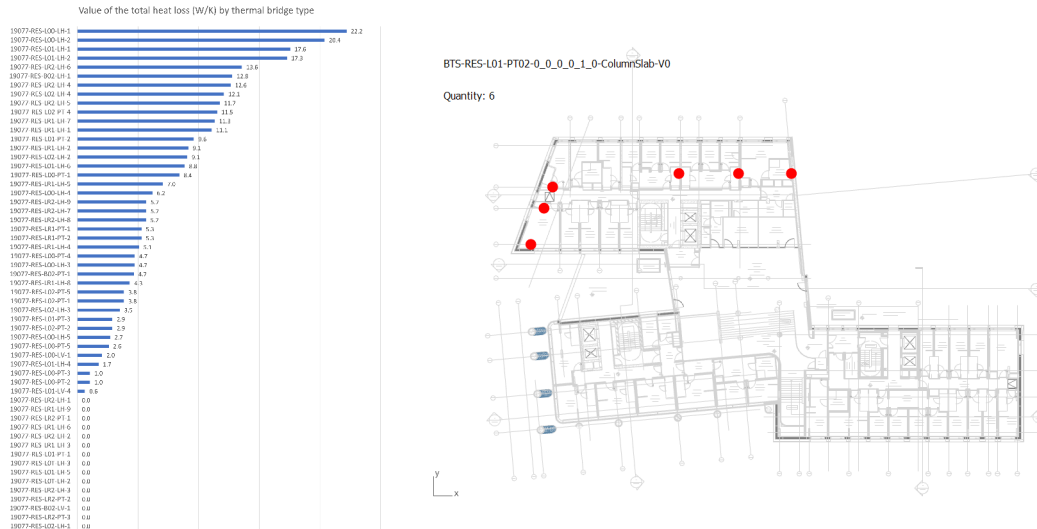
FIG. 8 Expected output for the two projects investigated. Left: summary of total heat loss per each thermal bridge. Right: example of the location of a thermal bridge in plan view (courtesy of Allford Hall Monaghan Morris).
