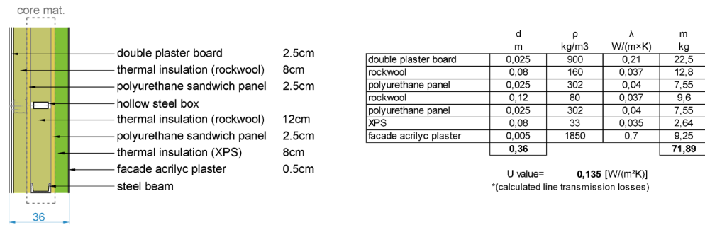
FIG. 14 Exterior wall system S8
