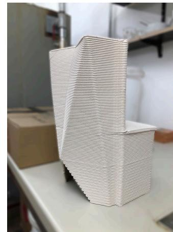
FIG. 13 Fired ceramic tile with a nest
