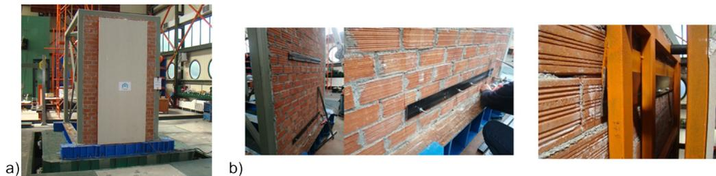
FIG. 6 Structural performance test of SmartWall: a) the experimental set-up and b) the anchoring system
