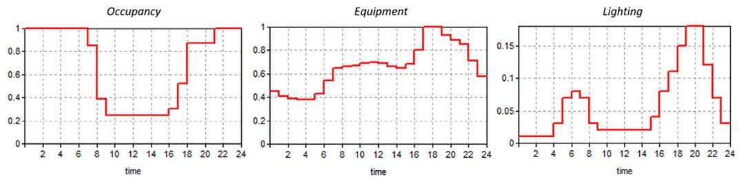
FIG. 13 Hourly profiles for occupancy, equipment and lighting
