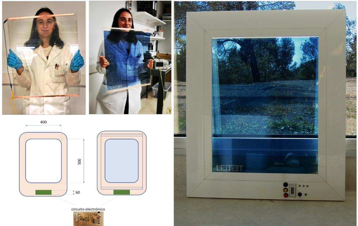
FIG. 12 (a), (b) and (c) are photos of the 45x50 cm<sup>2</sup> PLSMC prototype module realized in the frame of the INFINITE project. (d) Represent a schematic drawing of the demonstrator embedding an ad-hoc implemented control circuit.
