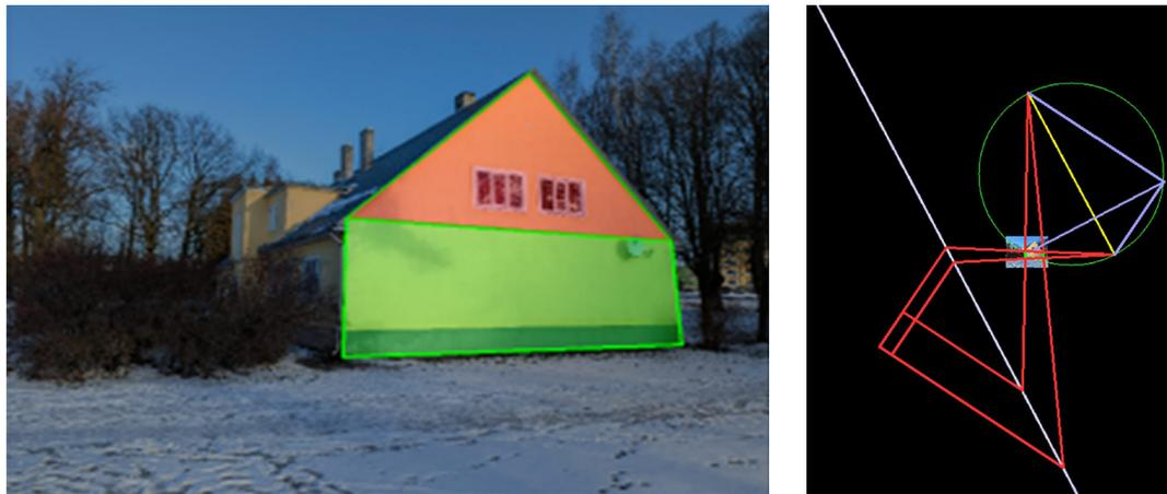
FIG. 5 Left, Tartu demo building façade with marked façade and gable area. Right, screenshot of the Python code, the algorithm for computing the height-width proportion from a façade image on the very same Tartu demo building
