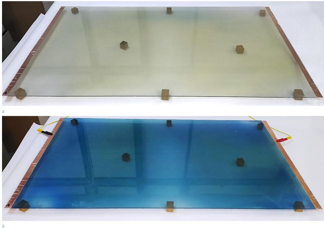
FIG. 4 70x130 cm<sup>2</sup> PLSMC module respectively in the a) WARM and b) DARK state.
