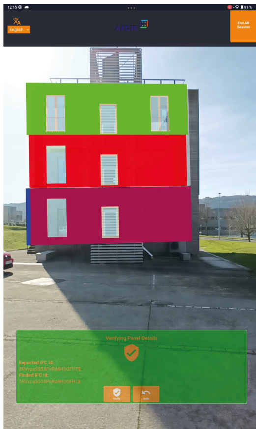
FIG. 18 Verified panels displayed in AR over the building.
