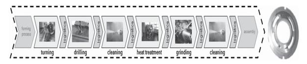
Fig. 3. Process chain for the production of a tax disc for hydraulic pumps, translation after Abele (2012).
